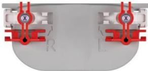
3 By opening the clasp slightly, the screws will fall securely into the screw guide and can then be installed in this position overhead in the upper window rebate as well.
