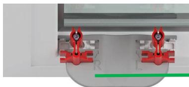
5 When the screw is firmly tightened, slide the fitting template down from the tension shoe to the centre of the window.
