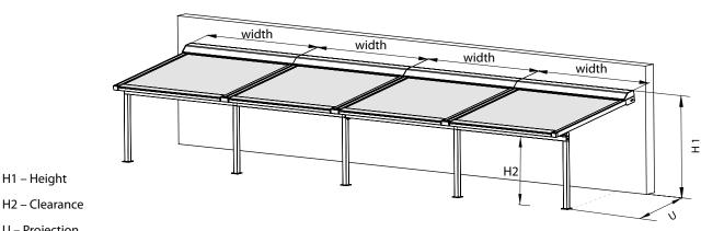
Note: In coupled systems, the intermediate stands are always fixed directly below the central guide rail.
