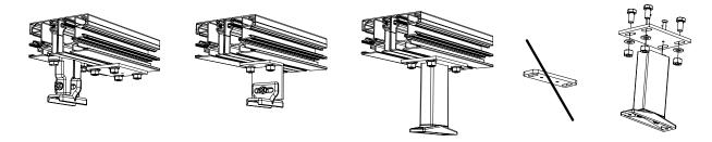
Bracket placed under the left or right guide rail Standard bracket placed in the middle
