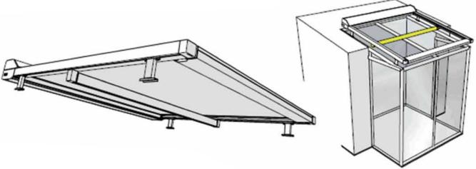
The support profile is always installed in a fixed position, in the center of the guide rails.
