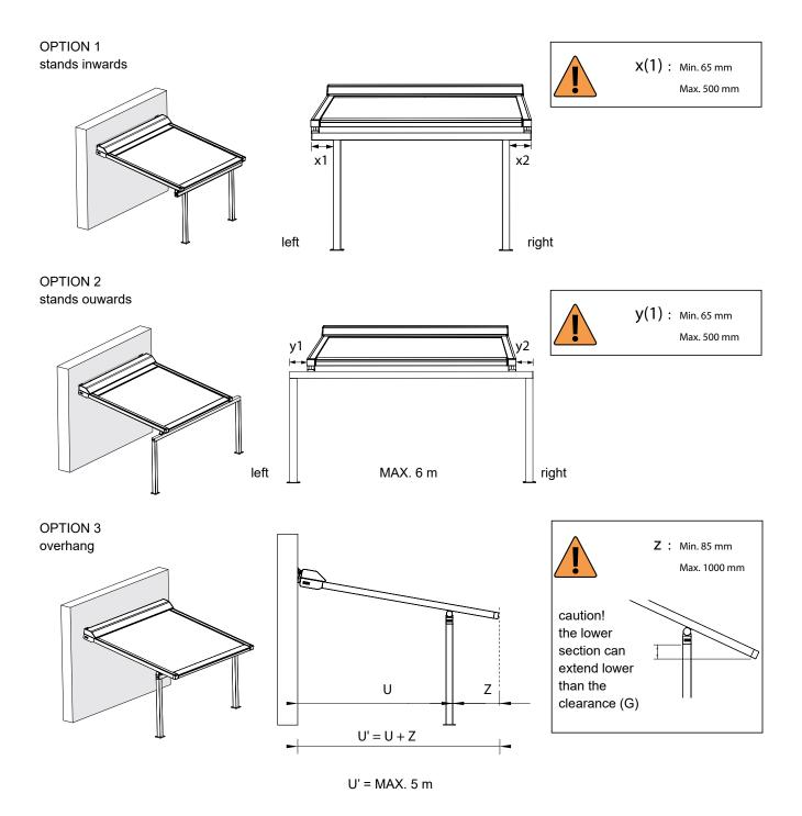
Make sure it is possible to open the box and lower section at all times to provide access to the mechanical parts inside. If this rule is not followed, ISOTRA cannot be held responsible for the cost of demolition work!
