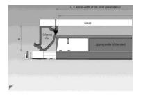
The ideal measurements of the blind are in the diagram. Such measurements can be taken by using the cut of the upper profile, the side board; by placing this aid on the glazing bar, it is possible to measure the point, maximum possible width of the blind and from this point the dimension of the same point on the opposite side is measured. This marking is always influenced by the form and size of the glazing bar of the window profile.
