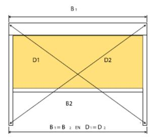
distance between guide rails = box width - 80 mm
