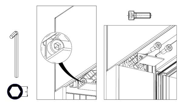
Halfway down, make a rotating movement to release the slide module from the guide rails.
