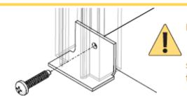
Please note that there is a hole in the bottom of the adjustment profile. Place the supplied end cap here, between the screw and the profile. Tighten everything to the window with screws.
