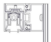
ENSURE THAT THE NOTCH IN THE GUIDE RAIL IS ALWAYS AT THE TOP (against the box)!
