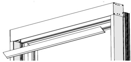
Remove the cover from the lateral guide. This is held in place by clips.
