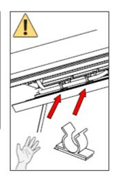
Remove the base plate. This is still connected to the box with a hinge.
