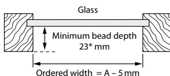
Due to possible dimensional tolerances of the windows, measure dimension A (width) in several places (points).
