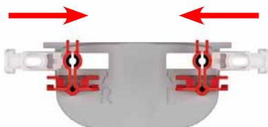
1. Push the lower parts of the tension shoe on the left and right into the recess on the side of the installation aid or press them in from below.
