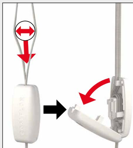
**All cord-operated blinds are supplied with a safety cord link which opens when the cord is spread to 60 mm and loaded with the weight under to 6 kg.**
