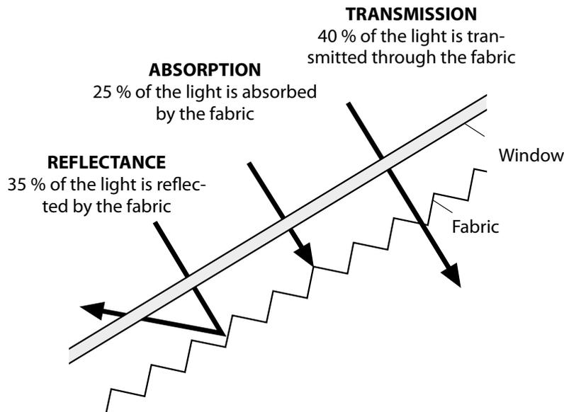
**Reflectance:** In the area of sun protection, reflectance is the percentage of incident sunlight that is reflected back to the outside directly or by diffusion. The more sunlight is reflected, the less percentage passes to the inner space to heat it.
