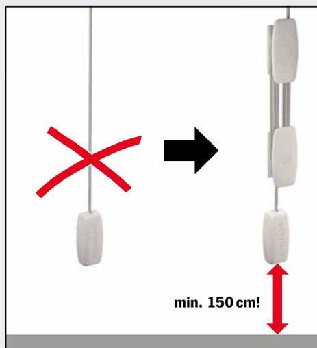
**In case of cord-operated blinds, it is absolutely necessary to install the cord winder.**
