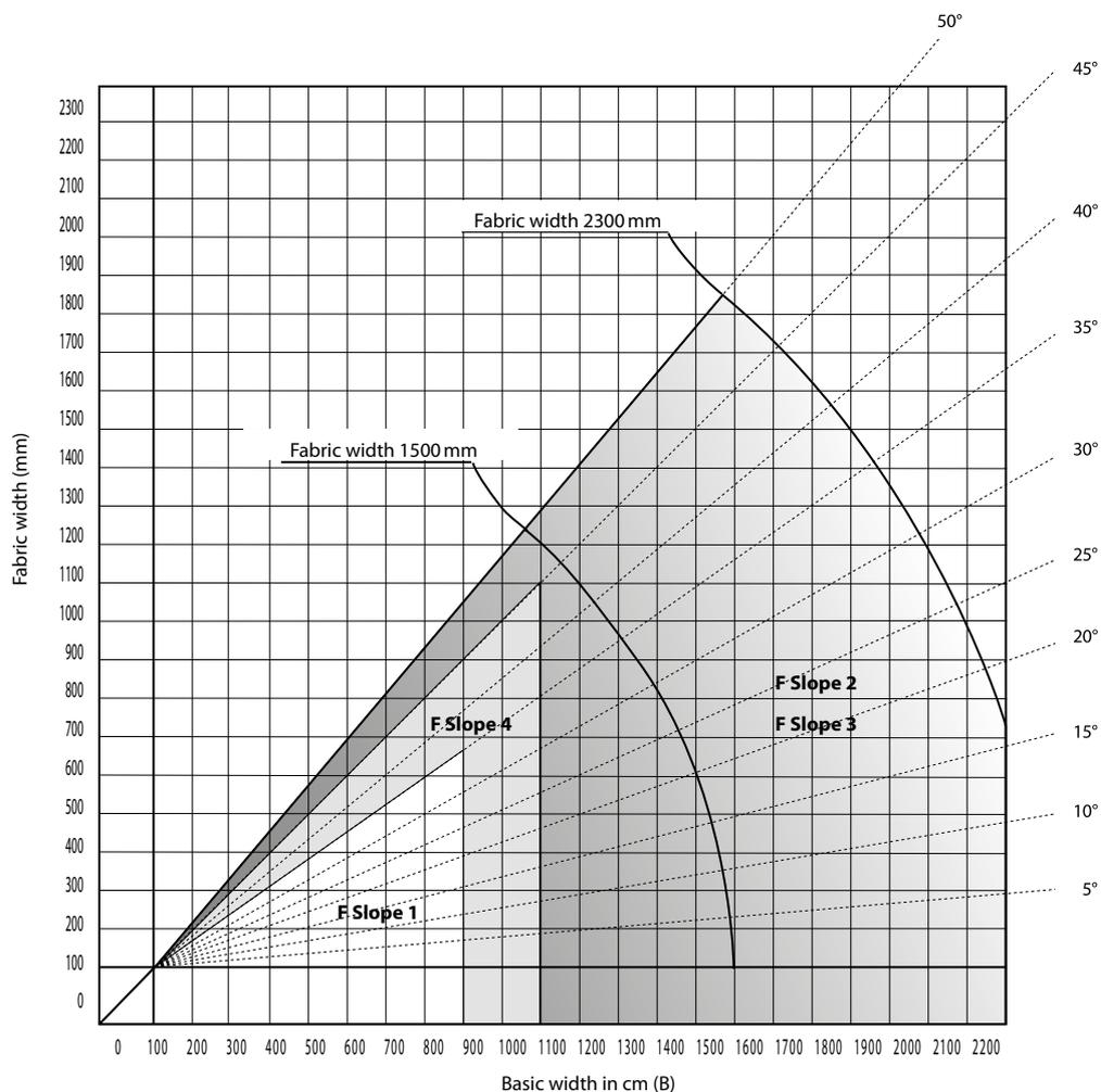
**The sharper is the angle, the smaller is the width.**
