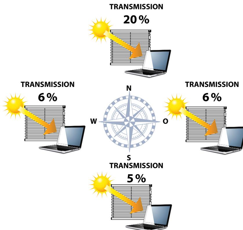
Shading of computer workplaces places high demands on glare protection, but it also must satisfy design and functionality requirements. Plisse blinds are best suited to this end. The blinds offer a wide range of control possibilities, they can be adapted to a variety of window shapes, and they provide long-lasting and high-quality solution of interior sun shading. This will eliminate or minimise annoying sun glare.
